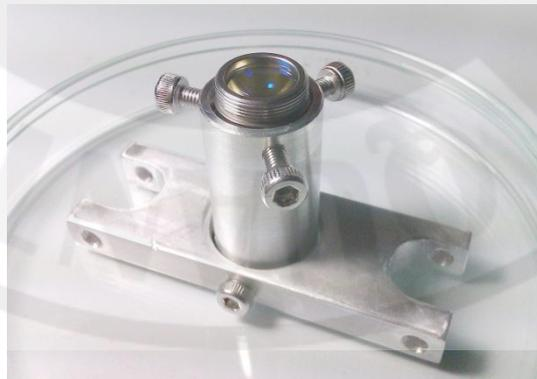
Figure 3.11: A homemade aluminium tube for clamping a high NA lens.
