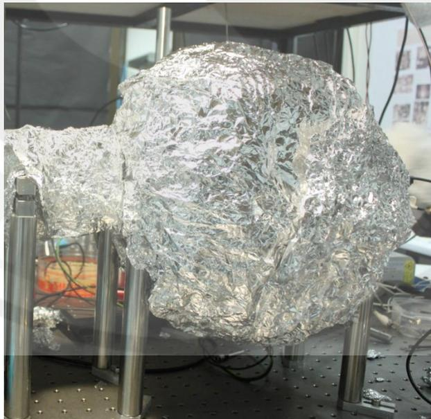
Figure 3.8: The chamber was covered with aluminium foil before baking process.
