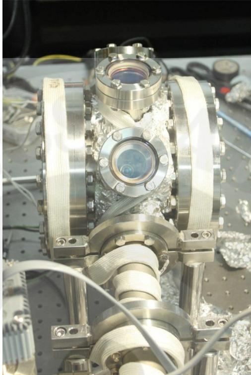
Figure 3.7: Two fiberglass heating tapes wrapped around 2 $\frac{3}{4}$ " and 8" viewports.
