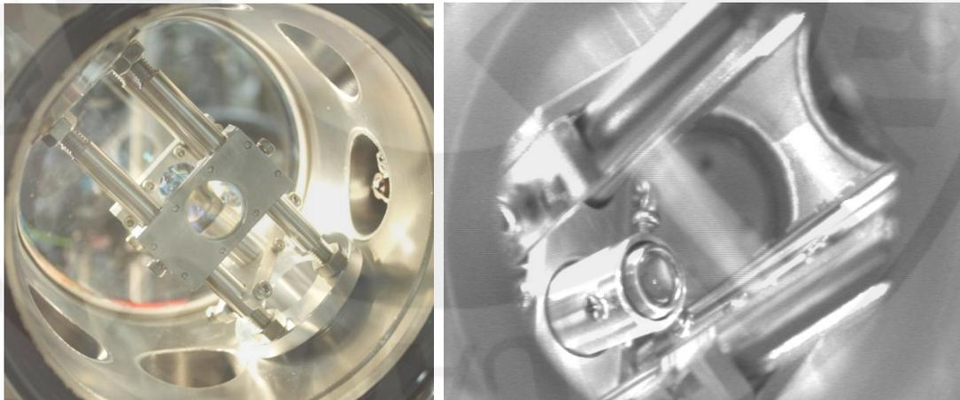
Figure 4.6: Shows the TBT setup. (left) Four straight rods and lenses were aligned by 45° degree from the vertical direction. (right) Small displacement of 50 mm lenses changed the direction of propagation of the laser beams and the beams were not completely overlapped.
